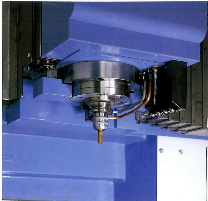
12000min<sup>-1</sup>{rpm} 仕様主軸
