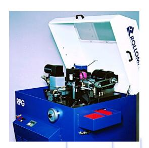
Easy access to all machine parts for quick setup and use. Compact with very low noise level. During operation, the totally enclosed grinding area allows for wet grinding to obtain higher quality surface finish. Tool diameter adjustments achieved in complete safety, without cycle interruption. User friendly instruction manual includes preventive maintenance information and mechanical/electrical prints.
